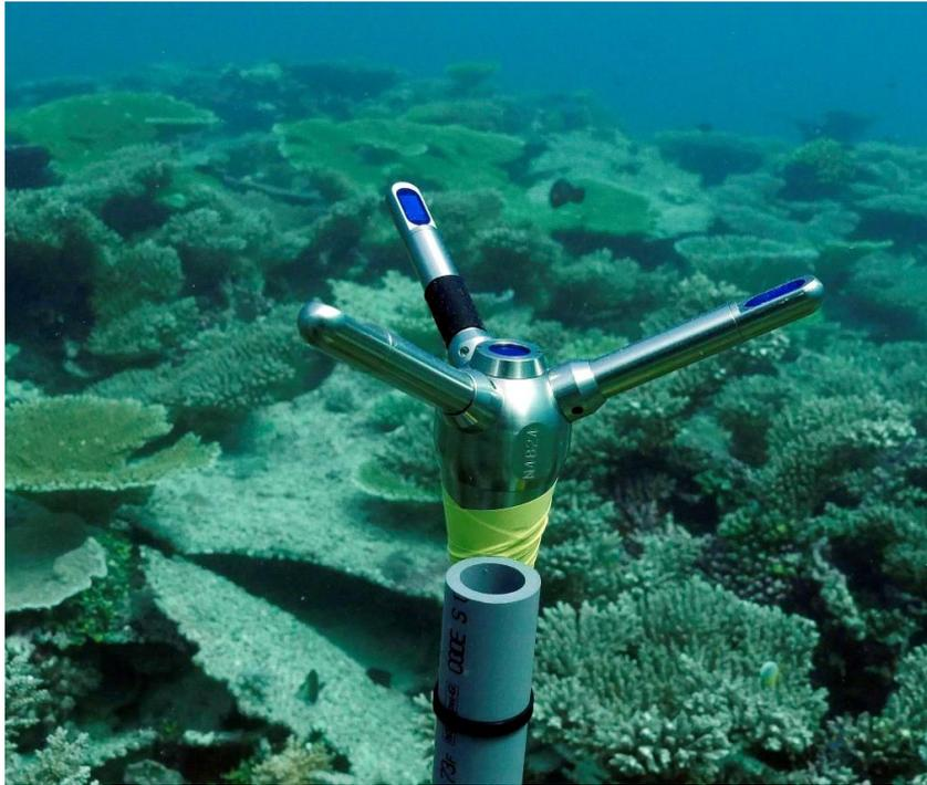
**Fig 19.** (left). We used Acoustic Doppler Velocimeters, such as this Vector instrument, to measure rapid small-scale changes in 3D velocity. This helps us understand turbulence and benthic boundary layer conditions.
