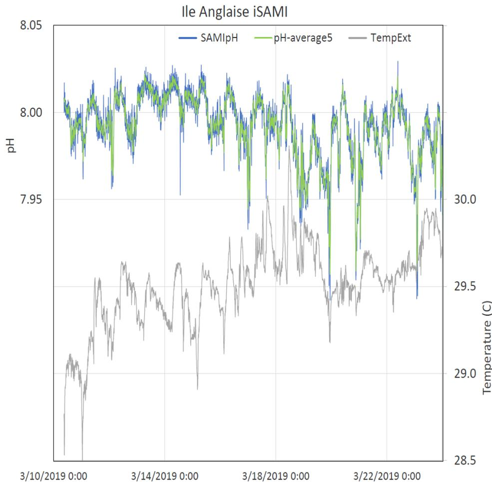
**Fig 21.** (left). pH and temperature recorded by a new design pH logger that exhibits both high precision and low drift during long ocean deployments. Diurnal variability is seen in pH as the community exhibits large changes in both primary production and carbonate formation, in this case forced by the day/night cycle.
