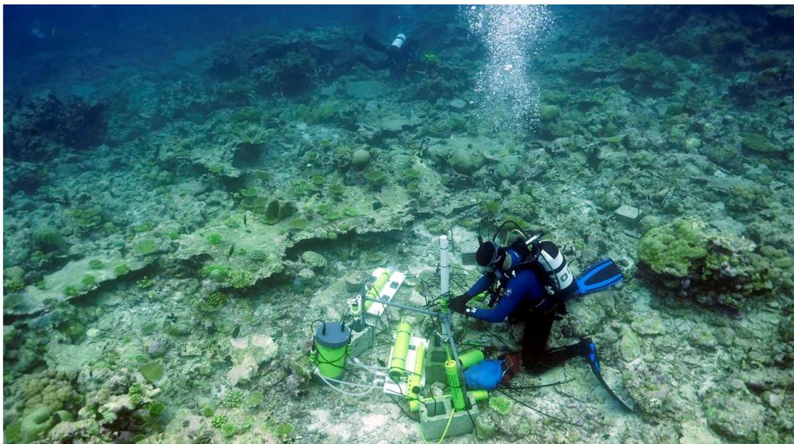
**Fig 20.** (above). Benthic flux measurement system deployed at Ile Anglaise from March 10-24, 2019. The basic setup was similar to that shown in Figure 4 but included an additional 6 instruments with new technology pH loggers, a direct pCO<sub>2</sub> logger, multiple oxygen loggers, a thermistor chain, and several kinds of high precision current meters. An Acoustic Doppler Current Profiler (ADCP) was deployed for a year (2019-2020) and can be seen at the very top of the above photograph.
